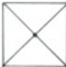
Detail #1 Determining Footer Drill Location on End of 4" x 4" Beam
